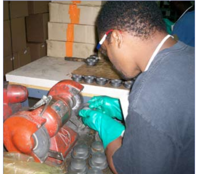
A client at SCVRD's Lancaster Work Training Center removes rust from parts for the ZF Commercial Suspension Systems and Components contract.
