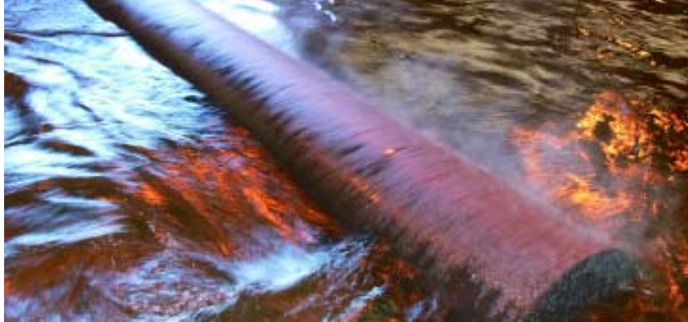
An extruded carbon electrode cools off in a water bath prior to being baked at temperatures up to 800 degrees Centigrade.
