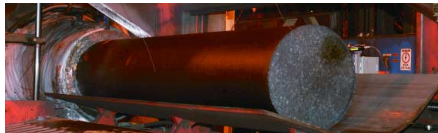
A carbon electrode is extruded and cut to length.
