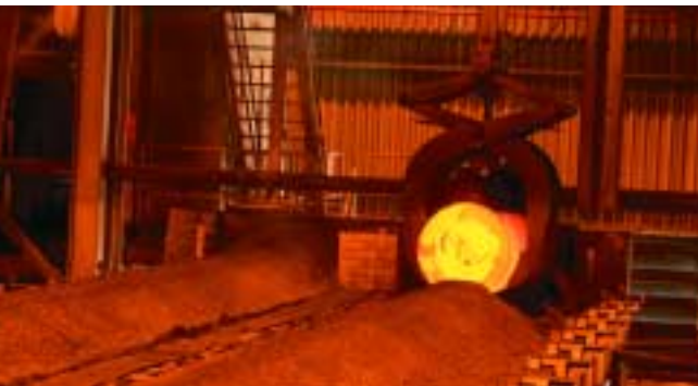
A red-hot electrode emerges from the electrically powered graphitizer furnace, which passes 120,000 amps of electricity through the electrodes for up to 20 hours.
