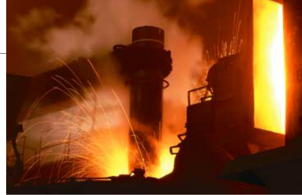
More than 140-million watts of Santee Cooper power flow through the carbon electrodes at Nucor Steel's plant in Berkeley County.
