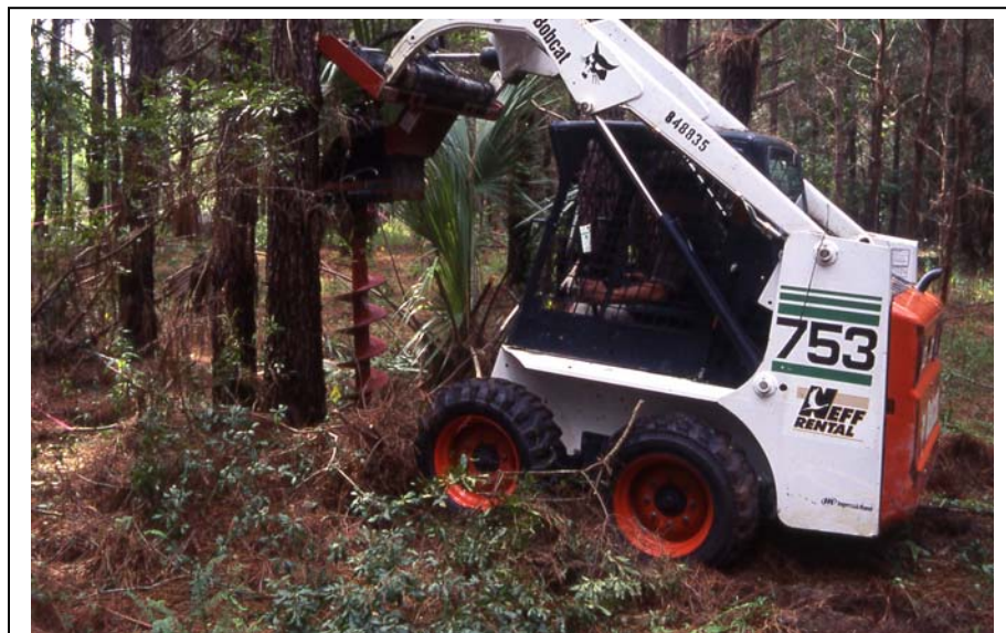
Figure 9. Use of Bobcat and 12-inch auger to conduct close interval tests.
