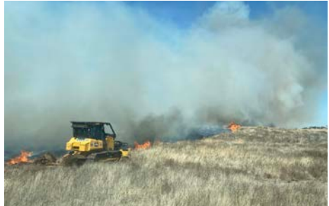
A dozer from Tennessee uses a lift plow to put in a line to contain the blaze.
