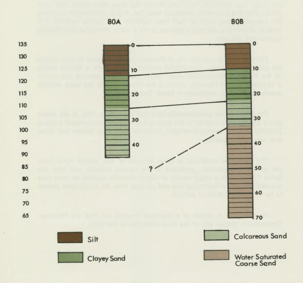
The site is underlain at a depth of approximately 65 feet by the Black Creek Formation, which is a dense black clay, with a bearing capacity of about 2,500-5,000 pounds per square foot (psf).
