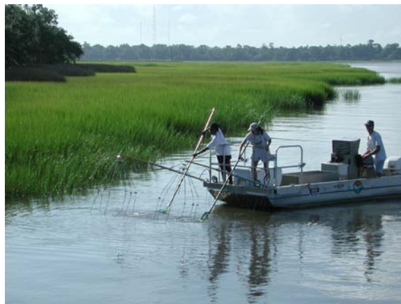
Fig. 1.6 SCDNR's Smith-Root electrofishing boat sampling fish in upper estuary habitat
