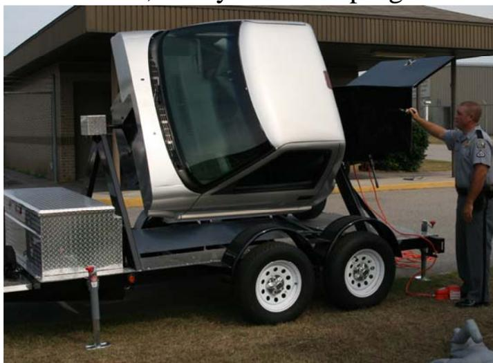
The Highway Patrol will introduce its Rollover Simulator this Fall. The simulator is meant to teach people about the effects of not buckling up, even at slow speeds. The Highway Patrol will use the simulator first in three counties with a high number of deaths involving lack of safety belt use: Lexington, Berkeley and Florence. It will eventually be used throughout the state.
